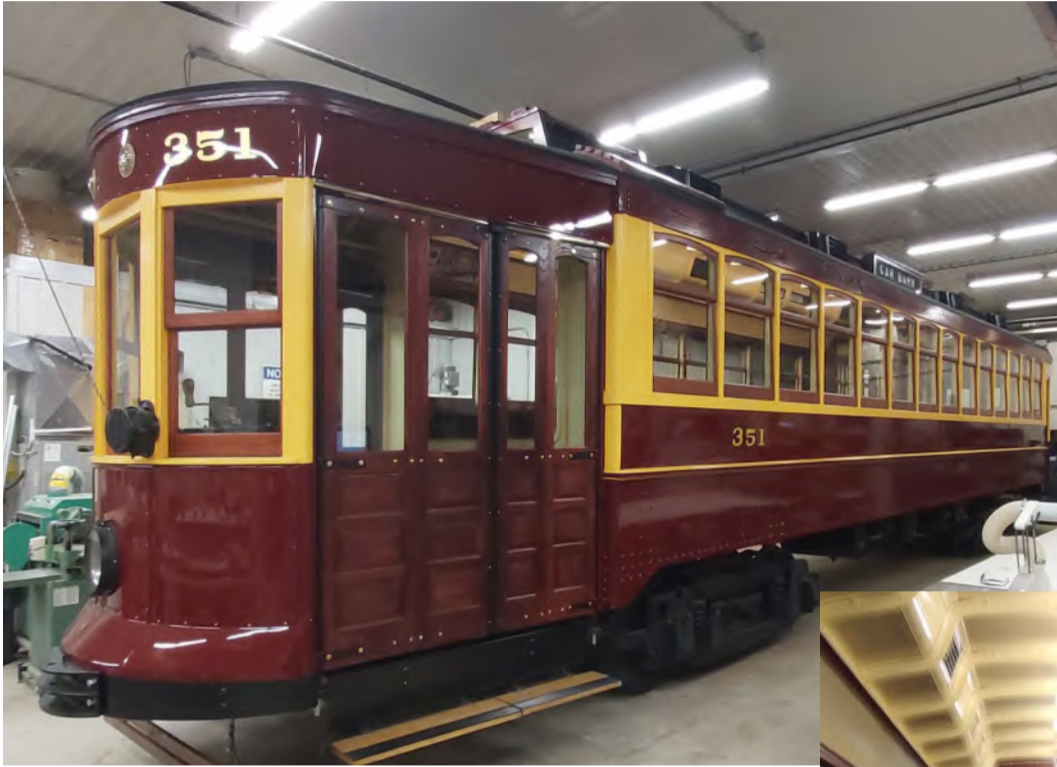
Top: SW&A streetcar #351 restored to like-new condition. The body was stripped down to the frame for a complete rebuilding which included the construction of a new floor and underside frame. The carbody was then reassembled with new parts where the original pieces were missing or beyond repair. Preparations are now underway to create a permanent indoor public space for this car.
