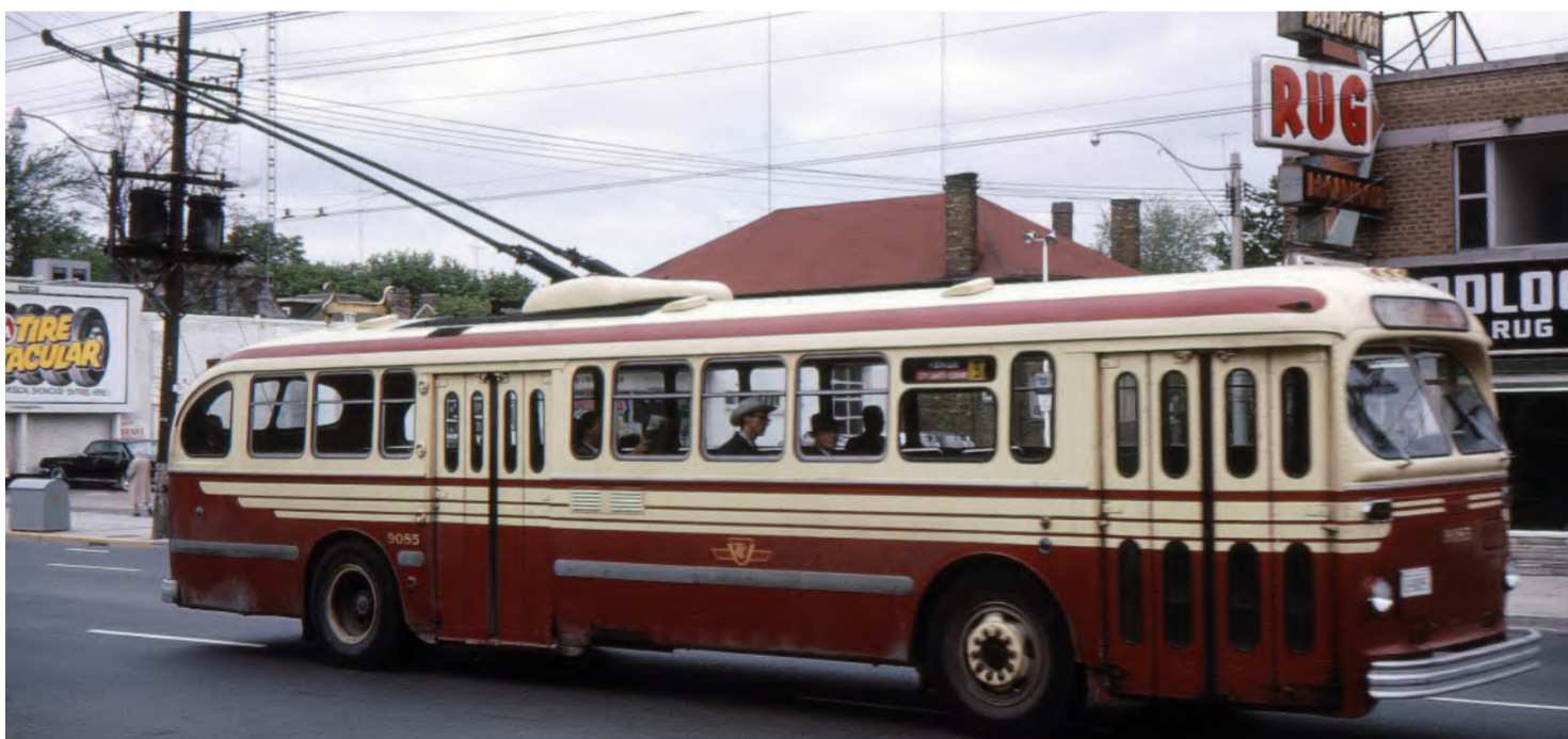
The final order of new T48A trolleys for the TTC consisted of 40 buses of a slightly different configuration. Using the flexibility of the Brill design these 40-foot buses were built with double-width front and rear doors, resulting in a slightly different side window arrangement on the right side (and probably 2 less seats). The 9085-9124 group would have been quick to unload at busy bus stops! Photo date: May 30, 1966. Photo: Peter Cox Collection via CTHF
