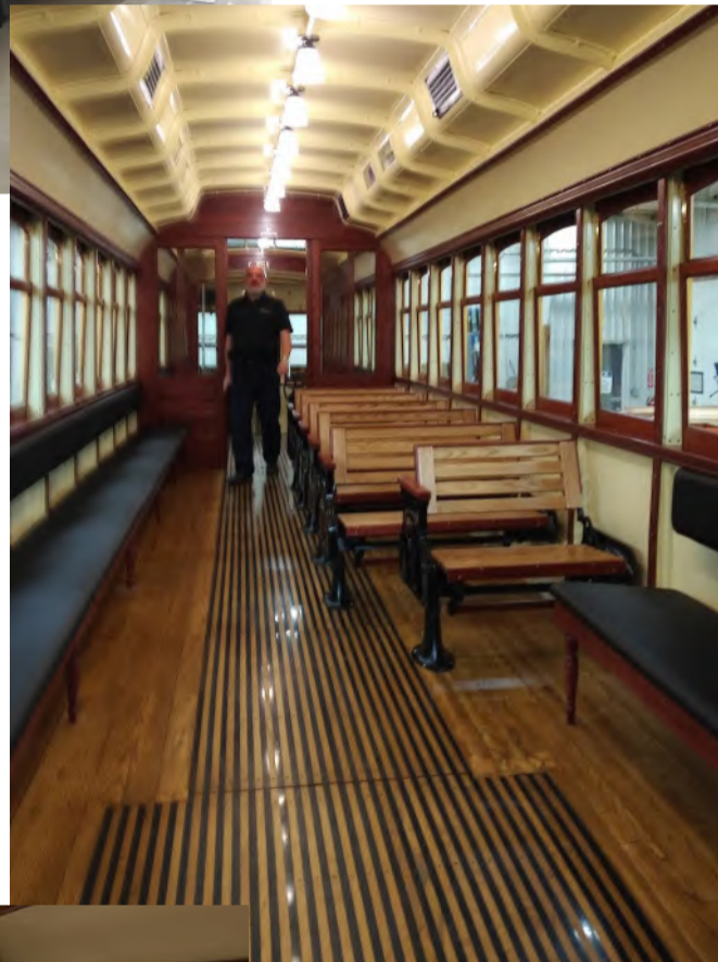
Top: SW&A streetcar #351 restored to like-new condition. The body was stripped down to the frame for a complete rebuilding which included the construction of a new floor and underside frame. The carbody was then reassembled with new parts where the original pieces were missing or beyond repair. Preparations are now underway to create a permanent indoor public space for this car.
